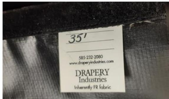
The curtain material was, “#L10KUP/DUP 10 oz vinyl coated polyester, inherently flame retardant”. This material is no longer available, and Drapery indicates that it was not intended for areas where lasers are being used. The product Drapery recommends is laser-rated at 250W/cm for 100 seconds and is certified in accordance with ANSI Z136.1-2007, Z136.7-2008, and NFPA-701. Even though the curtain looks like a laser safety curtain, it is not actually rated for safe use with lasers.
