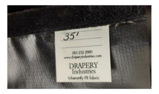
The curtain material was, "#L10KUP/DUP 10 oz vinyl coated polyester, inherently flame retardant". This material is no longer available, and Drapery indicates that it was not intended for areas where lasers are being used. The product Drapery recommends is laser-rated at 250W/cm for 100 seconds and is certified in accordance with ANSI Z136.1-2007, Z136.7-2008, and NFPA-701. Even though the curtain looks like a laser safety curtain, it is not actually rated for safe use with lasers.
