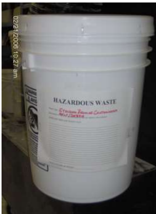
Figure 4 - Properly Labeled Plastic Bucket For Collecting Ethidium Bromide Contaminated Gels and Debris
