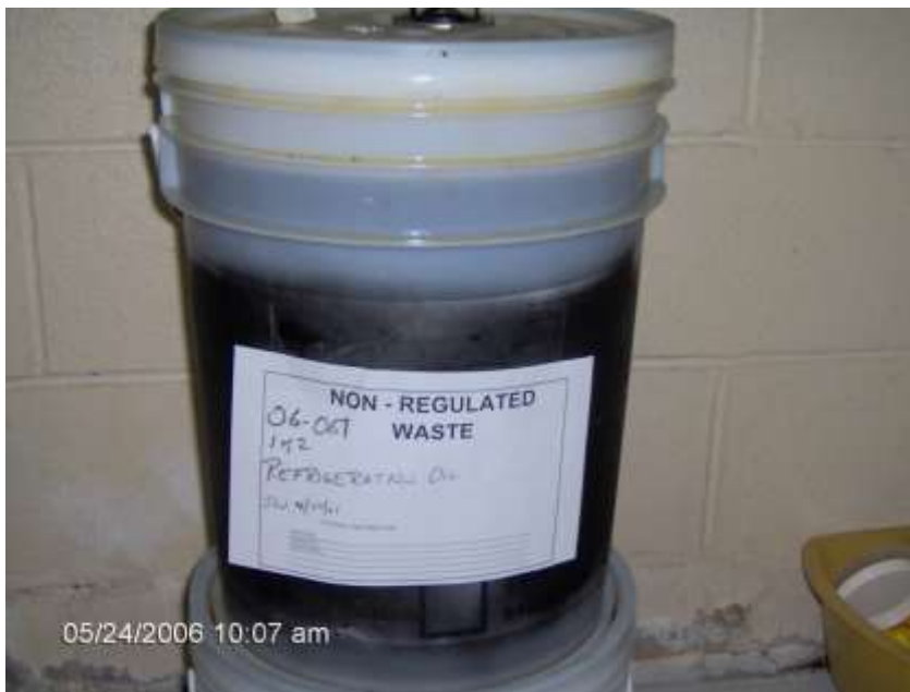
Figure 14 - Properly Labeled 5 Gallon Pail Containing Used Oil Contaminated With Refrigerants
